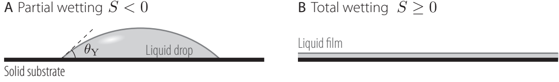
Figure 1.2 – A small drop is deposited on a planar surface and depending on the spreading coefficient S , it either adopts a spherical cap shape (as in A where S < 0 ) or it completely spreads and covers the surface (as in B where S \geq 0 ).
