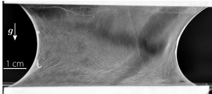
Figure 5.7 – Thick PAN membrane wicked with a large amount of water. Unlike the case presented in Figure 5.6, gravity now is oriented in the same direction as the compression axis of the membrane. This results in a wrinkling pattern where again, the preferred directions follow the circular arcs of the free edges. It should be noted that the inhomogeneities in the membrane’s color density correspond differences in thickness, but they do not affect the wrinkling pattern significantly.
